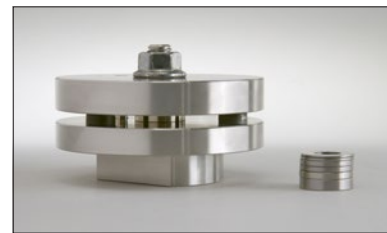
Compression Set Rig EV 03 , according to ISO 815-1.
