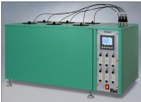
The EB 20 cell oven is equipped with 6 cells, each with individual temperatures.
