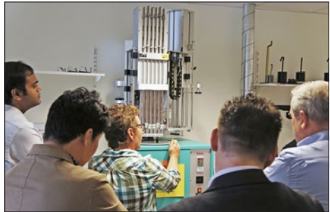
Mrs Ann-Cathrine Magnå demonstrates the Elastocon TR Tester, ET 01, in the combined instrument, which also includes a Gehman Tester, ET 02, and a Brittleness Tester, ET 05.
