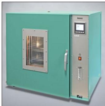
*Elastocon's cabinet ovens meet most ISO and ASTM standards for testing rubber and plastic materials. They can be equipped with a glass window and lamp, among other options.*
