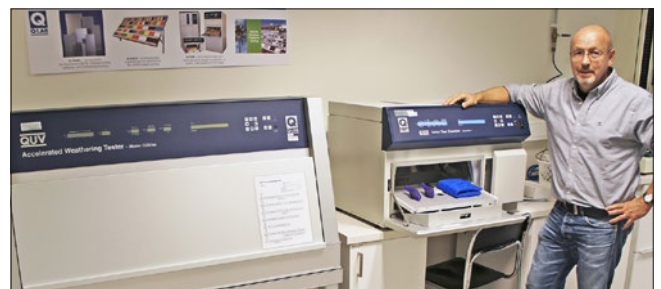
Pertti Steenari with the QUV Accelerated Weathering Tester, to the left, and the Q-SUN Xe-1 xenon arc chamber in Elastocon's testing laboratory.
