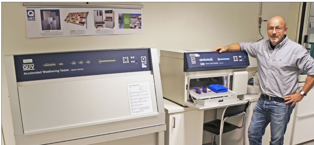
Pertti Steenari with the QUV Accelerated Weathering Tester, to the left, and the Q-SUN Xe-1 xenon arc chamber in Elastocon's testing laboratory.
